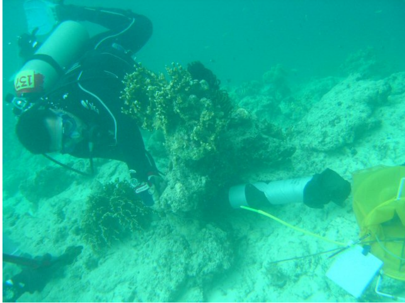
Figure 7 Cary McLean securing an SBE16 Conductivity and Temperature logger.
