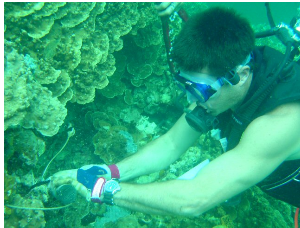
Figure 5 Cary McLean secures an SBE39 temperature logger to a coral outcrop using stainless steel wire.
