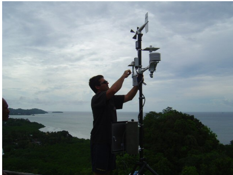
Figure 3 Portable Weather station being set up by Cary McLean.
